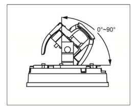
c. Remove the protective case by loosening the two screws on it before rotating the lens from behind.
