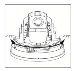
b. Tilt the lens after loosening the two screws on either side of the lens.
