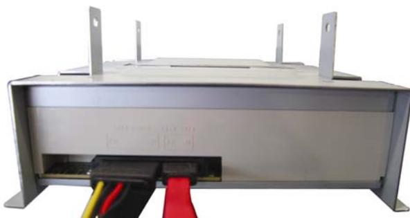
Step5: Replace the bracket to the DVR base and fix it.
