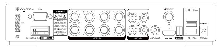
\* The VGA display will be off when the HDMI display is set to 4K2K
