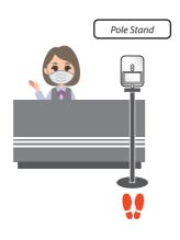
Install this tablet away from any direct heat / cold source, sun-facing window and significant airflow area as it may affect the stability of the room temperature and cause inaccurate temperature reading.
