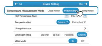
Each distance has different detection area. While choosing the distance, you can also check your face on the screen to see if a human face fits in the detection area and the temperature being taken is from the forehead.
