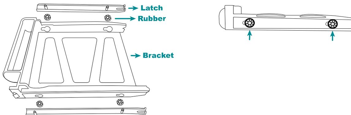
Step2: Get a compatible hard disk. With the PCB side facing down and the hard disk's connector facing the outside. Then, place the hard disk in the HDD tray and insert the latches.
